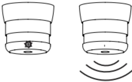
**Hush function:** In case of unintentional or false alarms, press and hold the hush button for 2 seconds (which is the entire bottom of the alarm). This will mute the alarm for 10 minutes, after which time the alarm will automatically resume its normal function.
