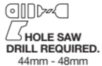
2. Using your hole saw (44mm-48mm), cut a hole into the surface. **CAUTION:** Ensure there is no wiring or any electrical equipment behind the surface you are drilling your hole into.
