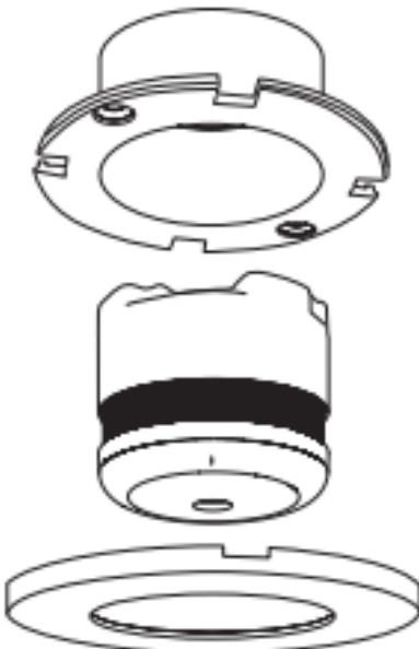
INSERT RECESS KIT MOUNTING BASE INTO THE HOLE AND SECURE WITH SCREWS
