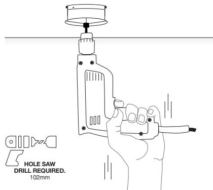
Screw recess kit base onto the ceiling. Then screw power supply unit inside the recess kit base.
