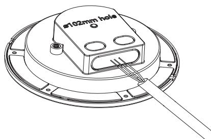
Connect the feed wire into the power supply unit and screw after termination.
