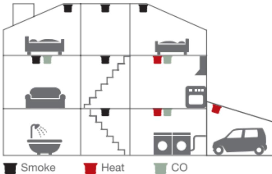
**Placement:** The thermal heat alarm is area specific. The alarm should be placed on the ceiling and near where the potential fire risks may occur.
