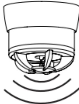
**Hush function:** In case of unintentional or false alarms, press and hold the hush button for 2 seconds (which is the entire bottom of the alarm). This will mute the alarm for 10 minutes, after which time the alarm will automatically resume its normal function.
