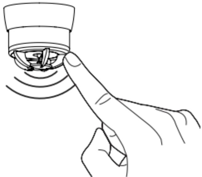
**Heat alarm signal:** The heat alarms have a visual and acoustic signal. In the passive state, the LED will flash every 48 seconds to indicate normal function. In alarming state the LED will flash and the alarm will emit a sweeping sound pattern designed to alert occupants.
