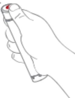
**Please note:** Due to coming legislation, the hush signal is transmitted with reduced power (the remote must be within short range from the silenced alarm, which means you should be in the same room as the alarm).
