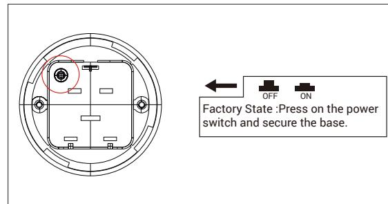
After installing the alarm, attach the alarm module back into the mounting base. Turn till you feel a click to ensure the alarm module is in to place.
